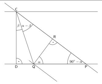
Fig. 2: Geometry of refraction of the laser.
