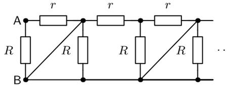
Everything apart from the two resistors which are closest to A is connected in parallel with a wire of zero resistance and therefore can be ignored. We are left with two resistors  $R$  and  $r$  in parallel which gives us the combined resistance as
