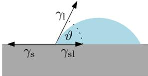
A droplet of water placed onto our mysterious material takes a steady axisymmetric form. In particular, this means that the horizontal components of forces along the line of contact must sum to zero. Mathematically, this is expressed by what is normally referred to as the Young's equation
