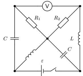
The properties of capacitors and coils are such that it is not possible to create a temporal discontinuity in potential difference across a capacitor and similarly with current through a coil. Therefore, after the switch is put off, there is a current  $I_2 = \varepsilon/R_2$  through the resistor  $R_2$ . Also, the current through the resistor  $R_1$  is now  $I_3 = I_2$ , so the potential difference across the two resistors is
